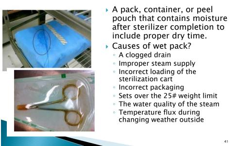
**Sterilization Process Failures**
